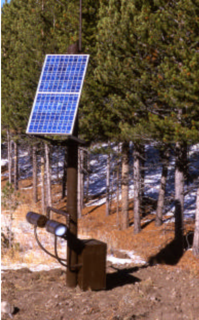
FIGURE 7 Solar powered animal sensors ( Photo courtesy of the Western Transportation Institute ).
